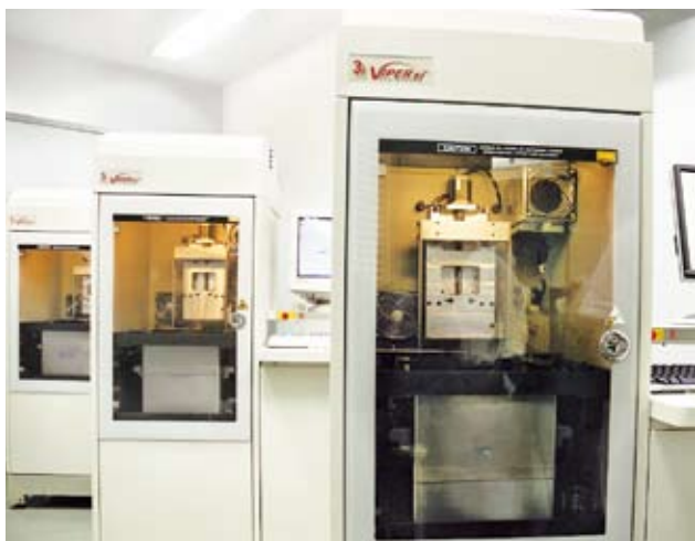
ViperSi2 a computer aided manufacturing machine
