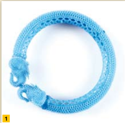
[1] Wax / rubber model in the first phase of CAD-CAM manufacture
